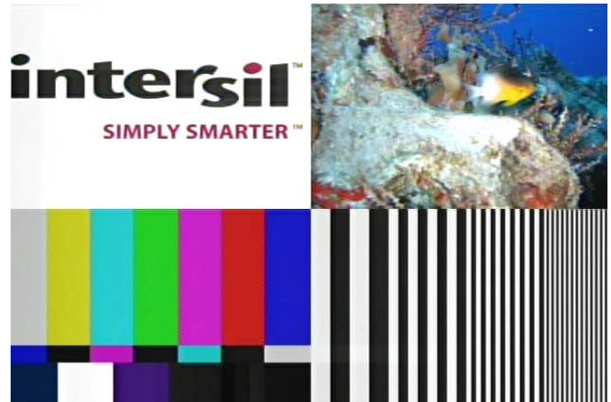
FIGURE 38. TEST PATTERN IMAGE AFTER 5000 FEET OF RG-59 COAX WITH ISL59603 (OR BETTER)
