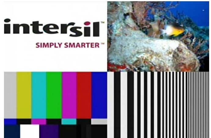
FIGURE 26. TEST PATTERN IMAGE AFTER 2000 FEET OF RG-59 COAX WITH ISL59602 (OR BETTER)
