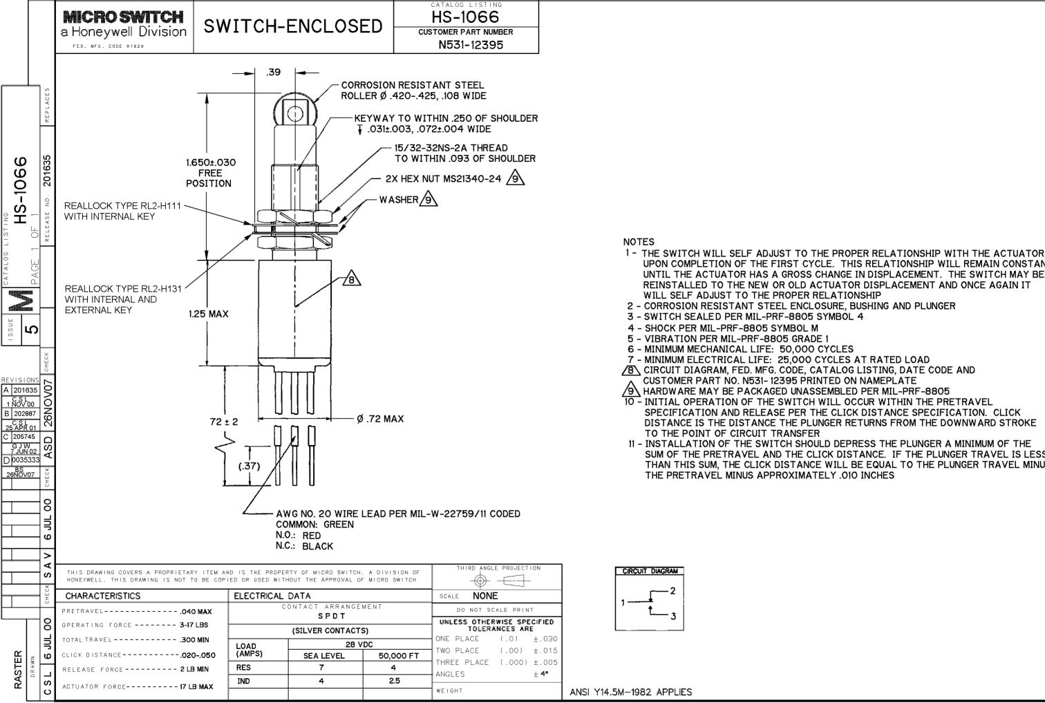
UPON COMPLETION OF THE FIRST CYCLE. THIS RELATIONSHIP WILL REMAIN CONSTANT UNTIL THE ACTUATOR HAS A GROSS CHANGE IN DISPLACEMENT. THE SWITCH MAY BE REINSTALLED TO THE NEW OR OLD ACTUATOR DISPLACEMENT AND ONCE AGAIN IT
