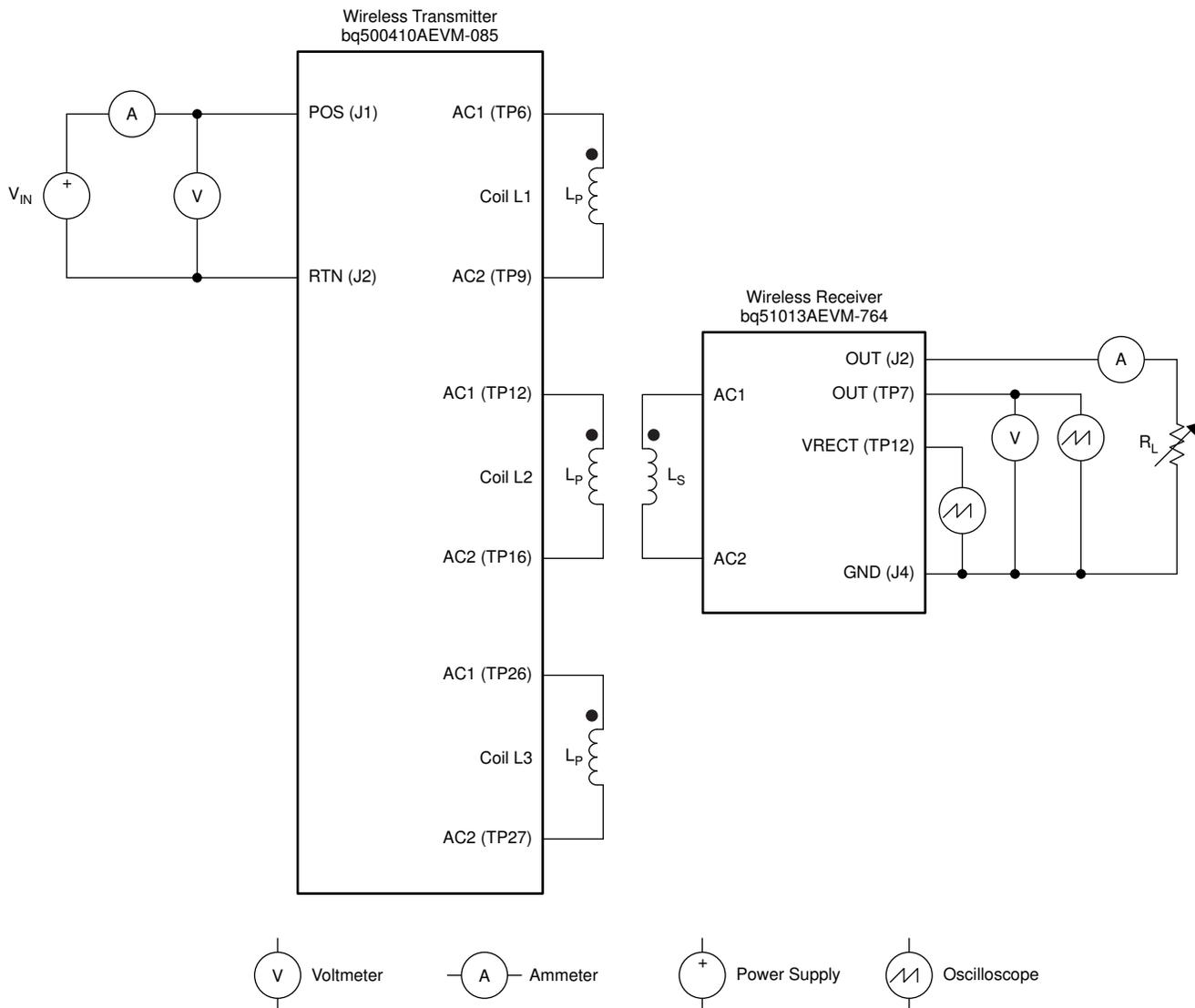
Figure 4. Equipment Setup
