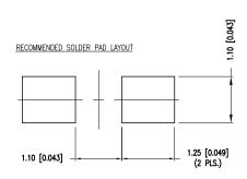
\*UNLESS OTHERWISE SPECIFIED TOLERANCES PER DECIMAL PRECISION ARE: X=±1 (±0.039), X.X=±0.5 (±0.020), X.XX=±0.5 (±0.010), X.XXX=±0.127 (±0.005). LEAD SIZE=±0.05 (±0.002), LEAD LENGTH=±0.75 (±0.030). MIN=  $\frac{+DECIMAL}{-0.000}$  PRECISION UNCONTROLLED DOCUMENT
