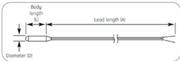
Designed for use in catheter assemblies, these sensors are available with nominal resistance values of 2252, 3000, 5000, and 10,000  $\Omega$  at 77°F (25°C). Close monitoring of manufacturing processes allow Thermometrics to maintain tight interchangeability tolerances with volume production. Typical design parameters are represented in Assembly Type table.
