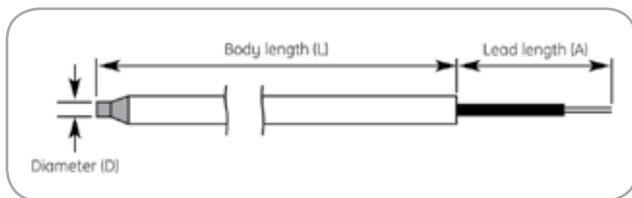
Intermittent body temperature measurements are common practice in all phases of patient care. This assembly is ideally suited for the disposable cover oral and rectal fever thermometers in use today. It features rugged construction with tip sensitive shaft assemblies exhibiting resistance values of 2252, 3000, 5000, and 10,000  $\Omega$  at 77°F (25°C). Refer to Assembly Type table for typical design parameters.
