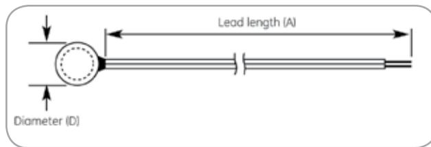
Routine continuous patient temperature monitoring is now feasible by using the convenience of the patient's skin site as an indicator of body temperature. The stainless steel housing used is suitable for both reusable and disposable applications, while maintaining maximum patient comfort. Nominal resistance values of 2252, 3000, 5000, and 10,000  $\Omega$  at 77°F (25°C) are available. Refer to Assembly Type table for typical design parameters.
