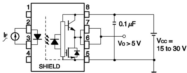
Fig. 6 UVLO Test Circuit
