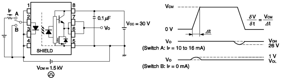
**Remark** CMR Test : Connect pin 1 and pin 4 to the LED common.
