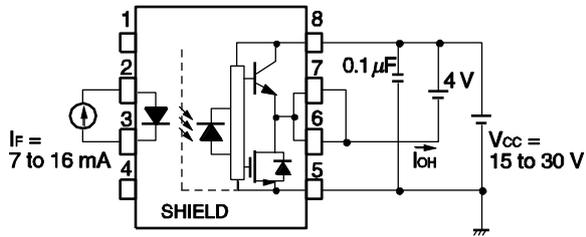
Fig. 2 I<sub>OL</sub> Test Circuit
