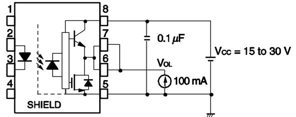
Fig. 5 I<sub>FLH</sub> Test Circuit
