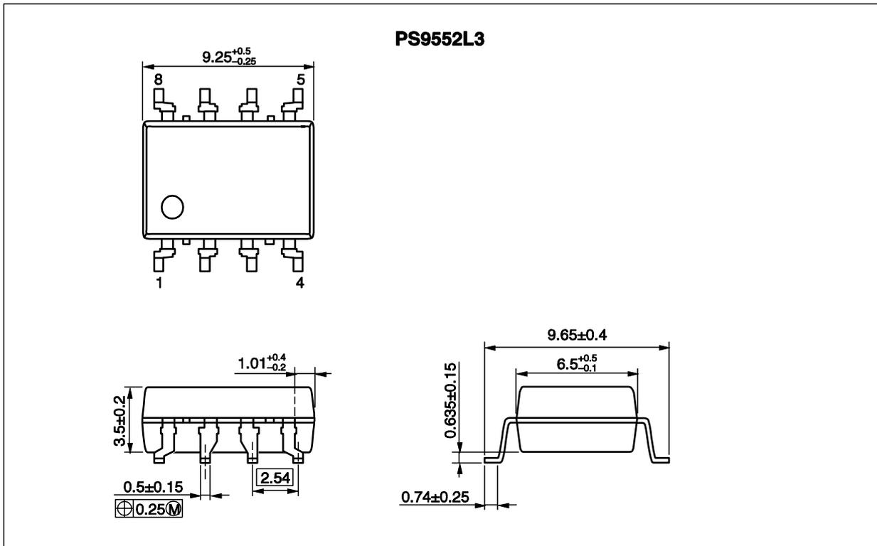
Lead Bending Type For Long Creepage Distance
