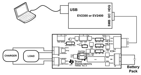
Figure 7. bq27441 Circuit Module Connection to Pack and System Load/Charger
