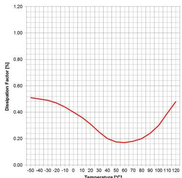
Temperature [°C] Test Equipment: E4991A or equivalent
