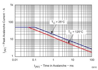
Figure 11. Single Pulse Unclamped Inductive Switching
