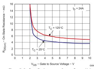
Figure 7. On-State Resistance vs. Gate-to-Source Voltage
