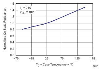
Figure 8. Normalized On-State Resistance vs. Temperature
