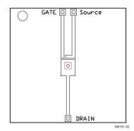
Max  $R_{\theta JA} = 162^{\circ} C/W$  when mounted on a minimum pad area of 2-oz. (0.071-mm thick) Cu.
