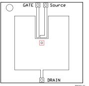
Max  $R_{\theta JA} = 58^{\circ} C/W$  when mounted on 1 inch² (6.45 cm²) of 2-oz. (0.071-mm thick) Cu.
