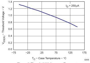
Figure 6. Threshold Voltage vs. Temperature
