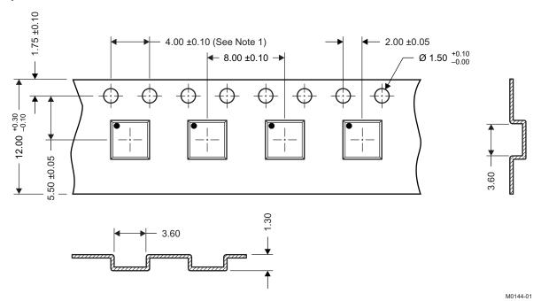
NOTES: 1. 10-sprocket hole-pitch cumulative tolerance ±0.2
