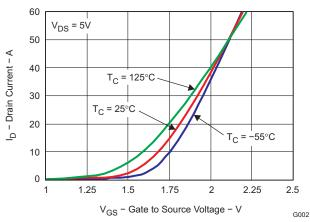
Figure 3. Transfer Characteristics
