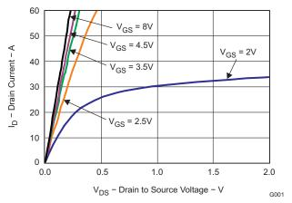
Figure 2. Saturation Characteristics
