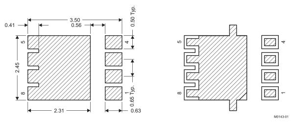
For recommended circuit layout for PCB designs, see application note SLPA005 – Reducing Ringing Through PCB Layout Techniques.
