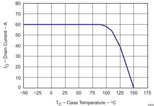
Figure 12. Maximum Drain Current vs. Temperature
