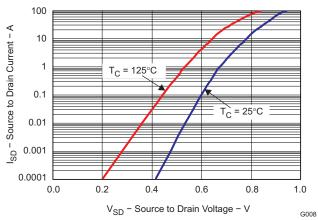
Figure 9. Typical Diode Forward Voltage
