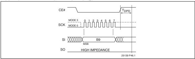
FIGURE 5-12: RELEASE FROM DEEP POWER-DOWN SEQUENCE
