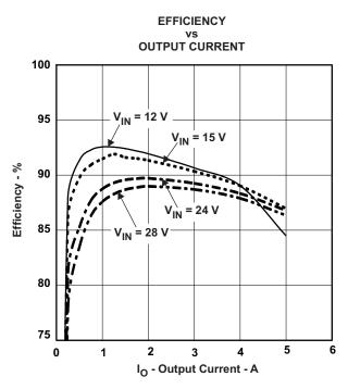
Figure 1. Measured Efficiency, TPS5450
