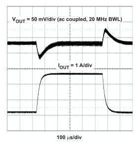
Figure 4. Load Transient Response, TPS5450
