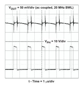
Figure 6. Measured Output Voltage Ripple, TPS5450
