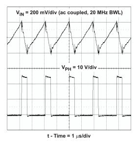
Figure 7. Input Voltage Ripple, TPS5450
