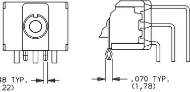
**AV1** VERTICAL RIGHT ANGLE, EXTENDED, PC THRU-HOLE, .150° PITCH
