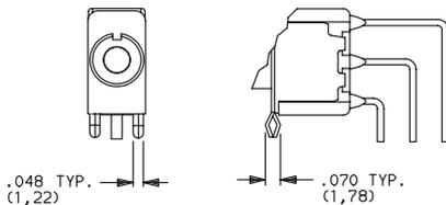
**AV1** VERTICAL RIGHT ANGLE, EXTENDED, PC THRU-HOLE, .150" PITCH
