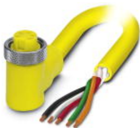
Sensor/actuator cable, 5-position, PVC, yellow, free cable end, on Socket angled 7/8"-16UNF, A-coded, cable length: 4 m
