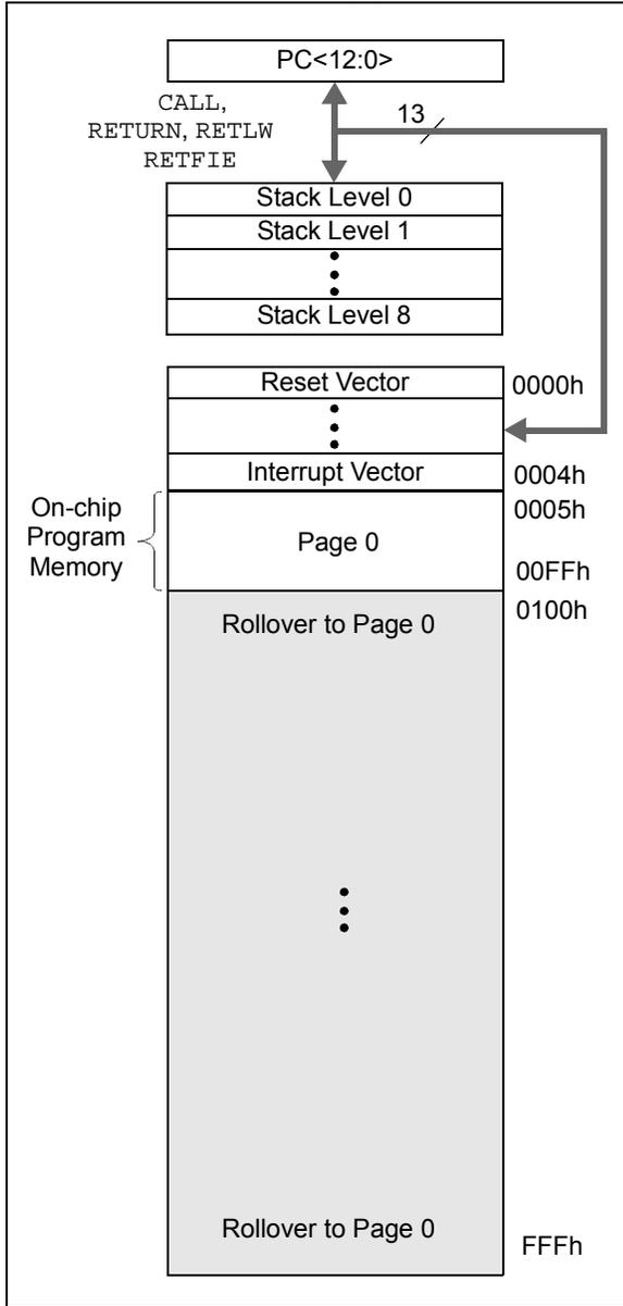
**FIGURE 2-2: PROGRAM MEMORY MAP AND STACK FOR PIC10(L)F322**
