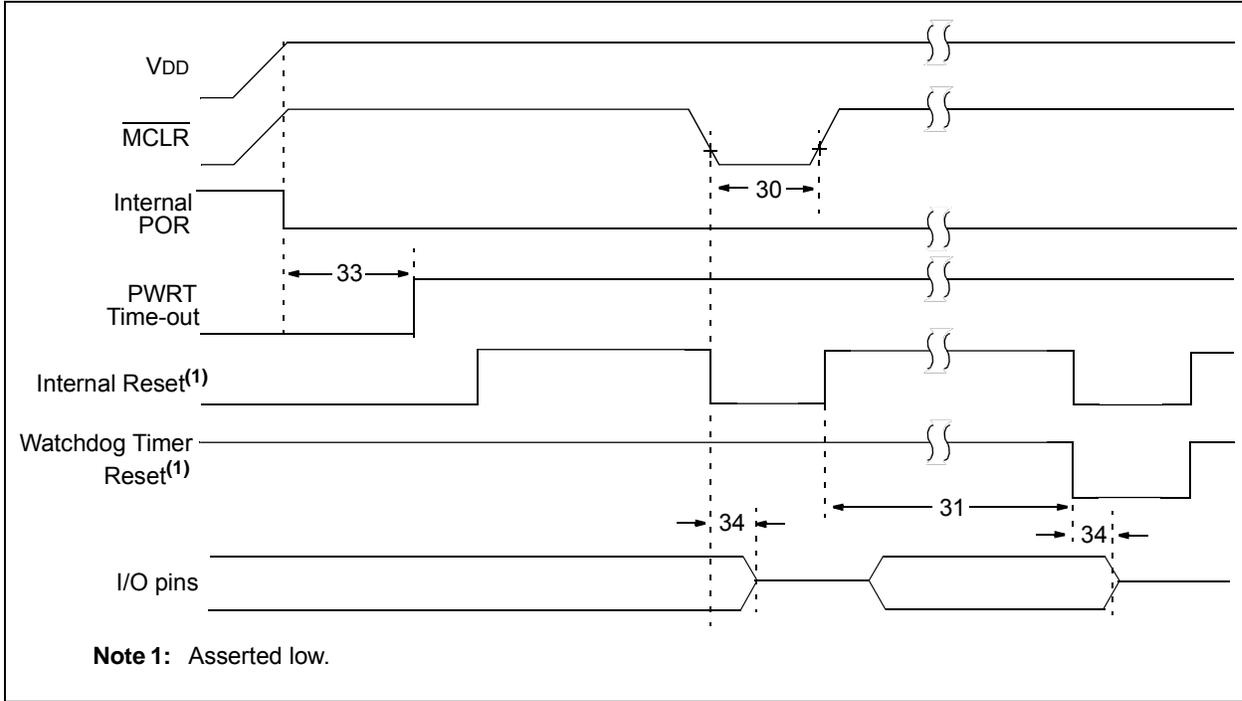
**FIGURE 24-9: BROWN-OUT RESET TIMING AND CHARACTERISTICS**
