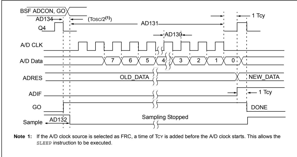
**FIGURE 24-13: A/D CONVERSION TIMING (SLEEP MODE)**
