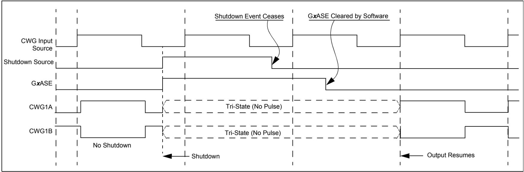
**FIGURE 21-6: SHUTDOWN FUNCTIONALITY, AUTO-RESTART ENABLED ( $GxARSEN = 1$ )**
