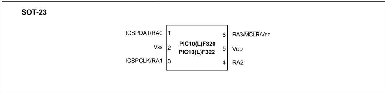
**FIGURE 2: 8-PIN DIAGRAM, PIC10(L)F320/322**
