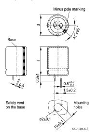
Snap-in terminals, length  $(6.3 \pm 1)$  mm. Also available in a shorter version with a length of (4.5 - 1) mm. PET insulation is marked with label "PET" on the sleeve.
