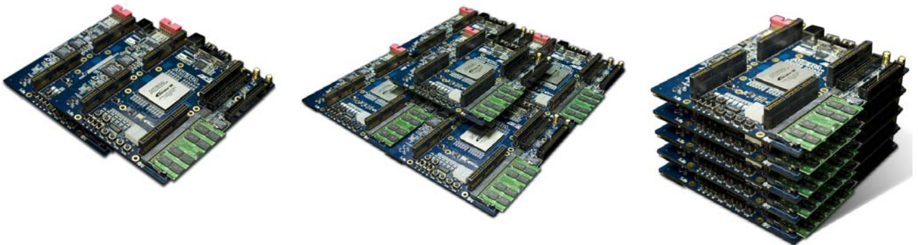
Figure 1.1 The stackable mechanism of the DE3 board
