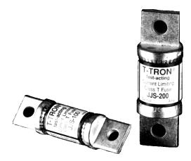
Catalog Symbol: JJN Current Limiting Very Fast Acting Ampere Rating: 1 to1200A Voltage Rating: 300Vac (or less)\* Interrupting Rating: 200,000A RMS Sym. Agency Information:
