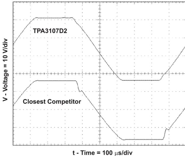
Figure 25. 1-kHz Sine Output at 10% THD+N
