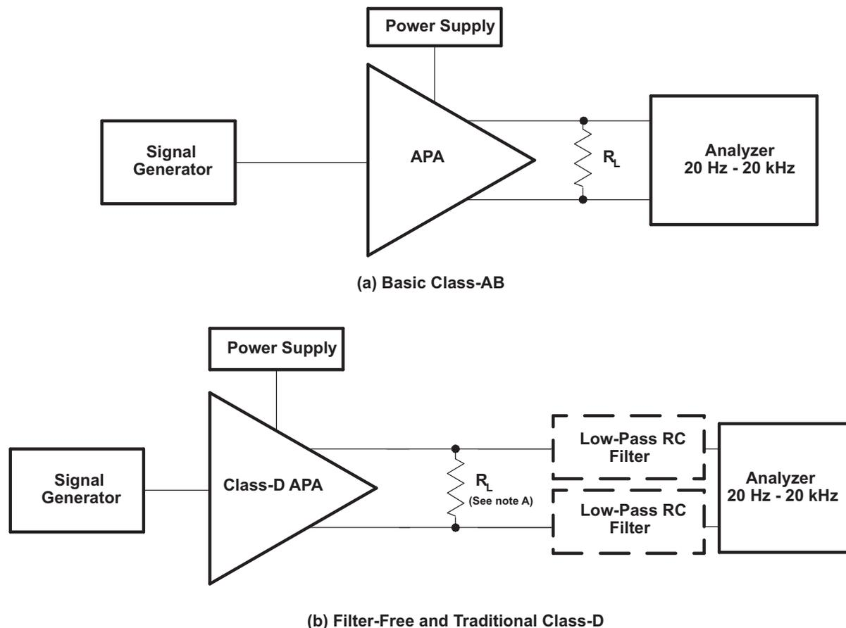
A. For efficiency measurements with filter-free Class-D,  $R_L$  should be an inductive load like a speaker.
