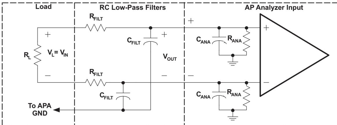
Figure 30. Measurement Low-Pass Filter Derivation Circuit-Class-D APAs
