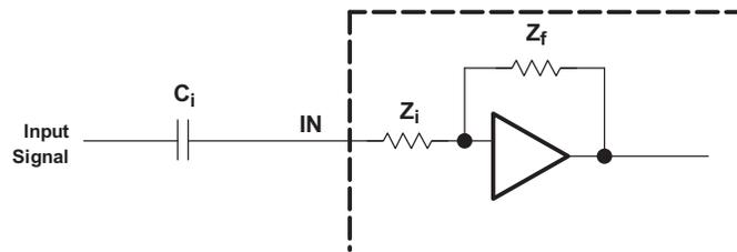
The -3-dB frequency can be calculated using Equation 1. Use the  $Z_i$  values given in Table 1.
