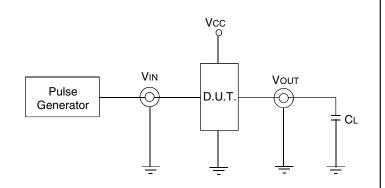
CL = Load Capacitance: Includes Jig and Probe Capacitance
