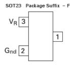
(Top View) Pin 1 floating or connected to pin 2
