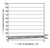
2.-(3) Electrical life test (90A type) (Resistive load 277V AC, 80A at 25°C 77°F)
