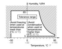
\* -50 to +85°C -58 to +185°F (When applied coil hold voltage is 50% to 60% of nominal coil voltage)
