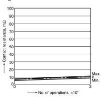
2.-(2) Electrical life test (48A type) (Resistive load 277V AC, 48A at  $85^{\circ}$ C  $185^{\circ}$ F)
