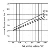
1.-(2) Coil temperature rise (48A type) Sample: HE1aN-P-DC9V-Y5, 6 pcs. Point measured: coil inside Ambient temperature: 25°C 77°F, 60°C 140°F, 85°C
