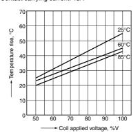
1.-(3) Coil temperature rise (90A type) Sample: HE1aN-W-DC12V-Y6, 6 pcs. Point measured: coil inside
