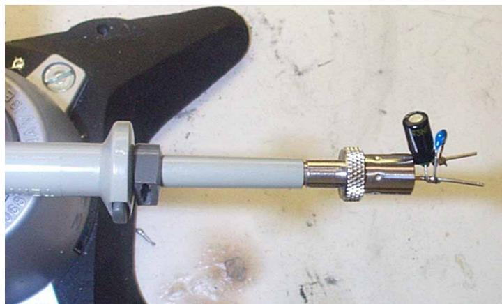
**Figure 31** – Oscilloscope Probe with Probe Master ([www.probemaster.com](http://www.probemaster.com)) 4987A BNC Adapter. (Modified with Wires for Ripple Measurement, and Two Parallel Decoupling Capacitors Added.)
