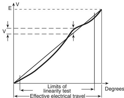
The independent linearity (conformity for the non-linear laws) is the maximum gap ΔV between the actual variation curve and the theoretical variation curve the nearest to it. The linearity and the conformity are expressed in percentage of the total applied voltage E
