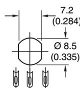
**BUSHING D AND E WITH LOCKING NUT**
