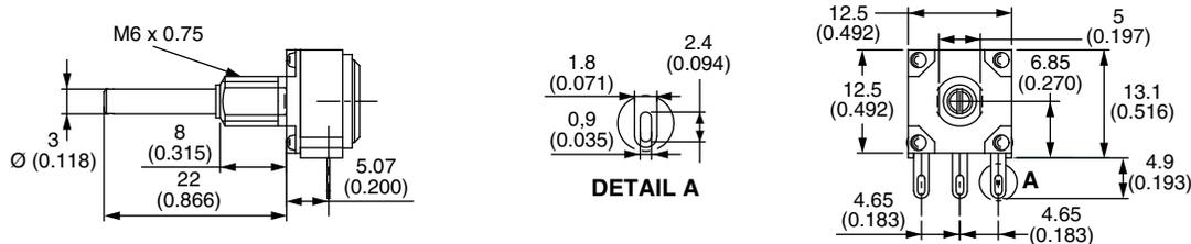
Single module, single shaft, vertical mounting, PC pins with support plate, metric bushing and shaft
