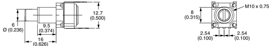
Dual modules, single shaft, PC pins with front support plates, imperial bushing and shaft
