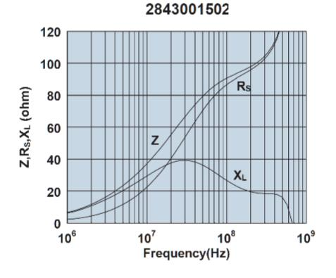
Impedance, reactance, and resistance vs. frequency.
