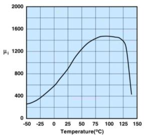
Measured on a 17/10/6mm toroid at 100kHz.
