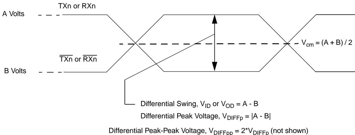
**Figure 37. Differential Voltage Definitions for Transmitter or Receiver**
