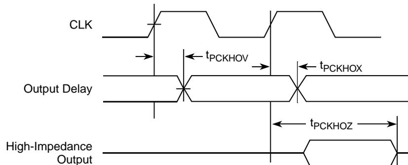
Figure 36. PCI Output AC Timing Measurement Condition
