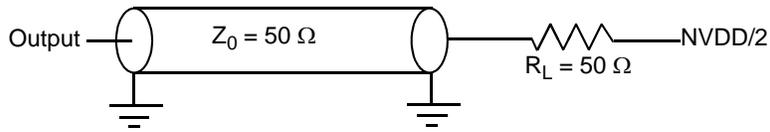
**Figure 27. AC Test Load for the JTAG Interface**
