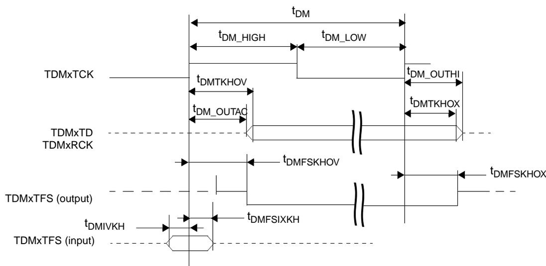
Figure 58. TDM Transmit Signals
