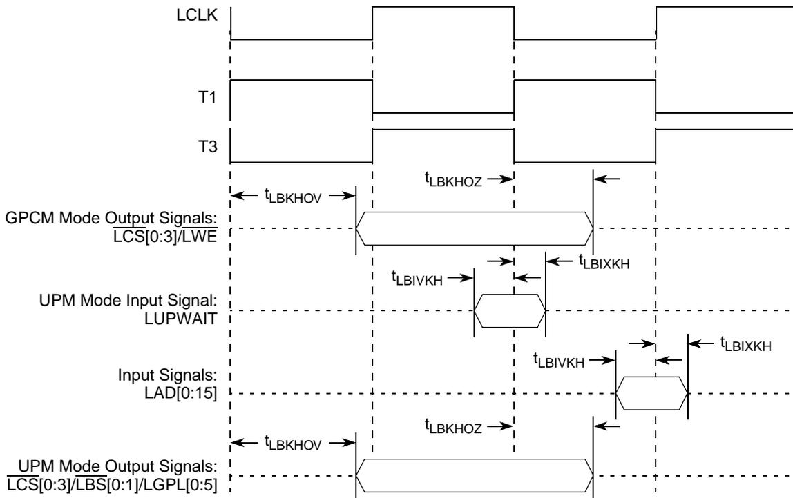
Figure 25. Local Bus Signals, GPCM/UPM Signals for LCRR[CLKDIV] = 2
