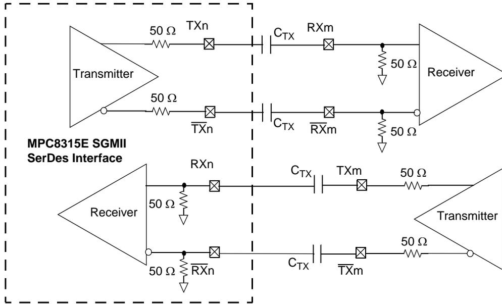
Figure 17. 4-Wire AC-Coupled SGMII Serial Link Connection Example
