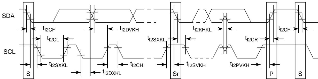
Figure 33. I<sup>2</sup>C Bus AC Timing Diagram
