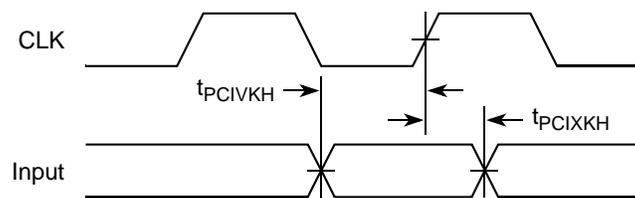
Figure 35. PCI Input AC Timing Measurement Conditions
