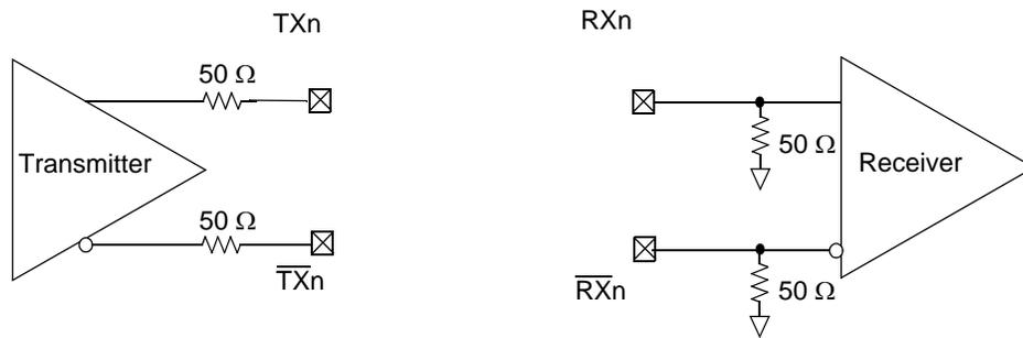
**Figure 48. SerDes Transmitter and Receiver Reference Circuits**
