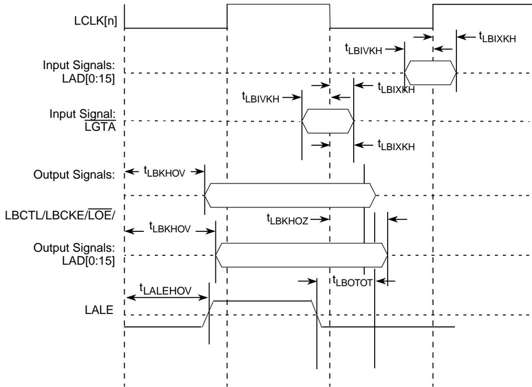
Figure 24. Local Bus Signals, Nonspecial Signals Only
