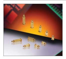
Single Pogo Pin contacts provide high cycle life in industrial and medical applications where reliability and robustness is critical. Pogo Pins provide 10,000 mating cycles and are ideal in pluggable module applications where the end customer has to handle a product daily. Pogo Pins are designed to mate with gold plated PCB pads or flat contacts in docking/cradle applications to function as the charging, data transfer or programming interface to a portable device.
