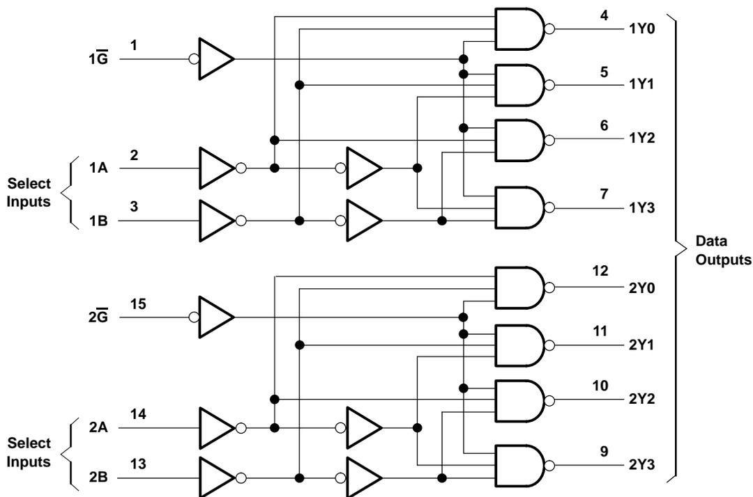
Pin numbers shown are for the D, DB, DGV, J, N, NS, PW, and W packages.
