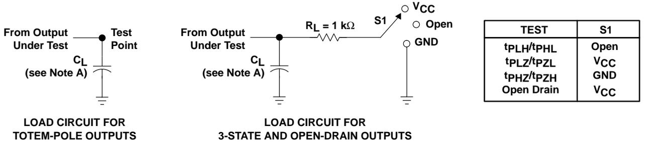
LOAD CIRCUIT FOR TOTEM-POLE OUTPUTS
