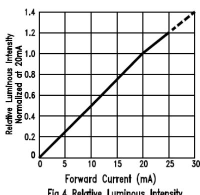
Fig.4 Relative Luminous Intensity
