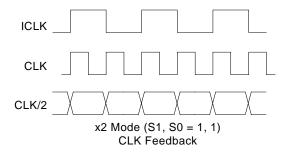
Using CLK as the feedback will always result in synchronized rising edges between ICLK and CLK. However, the CLK/2 could be a falling edge compared with ICLK. IDT recommends using CLK/2 feedback whenever possible. This will synchronize the rising edges of all three clocks.
