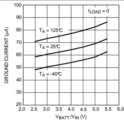
Figure 5. Ground Current vs  $V_{BATT} / V_{IN}$
