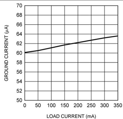
Figure 6. Ground Current vs Load Current
