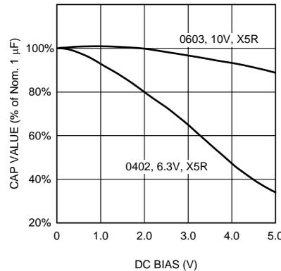
**Figure 10. Typical Variation In Capacitance vs DC Bias**
