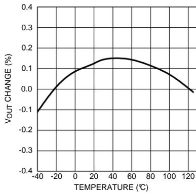
Figure 1. Output Voltage Change vs Temperature
