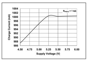
**FIGURE 2-6:** Charge Current  $(I_{OUT})$  vs. Supply Voltage  $(V_{DD})$ .
