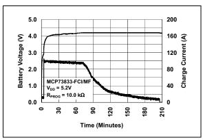
FIGURE 2-17: Complete Charge Cycle (180 mA Li-lon Battery).
