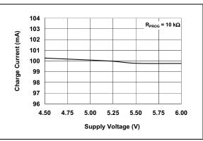
**FIGURE 2-5:** Charge Current  $(I_{OUT})$  vs. Supply Voltage  $(V_{DD})$ .
