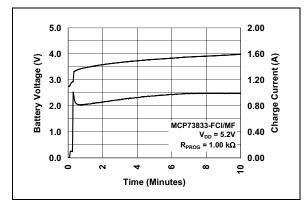
**FIGURE 6-3:** Typical Charge Cycle Start with Thermal Regulation (1700 mAh Li-Ion Battery).
