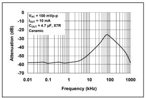
**FIGURE 2-11:** Power Supply Ripple Rejection (PSRR).
