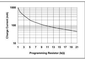
**FIGURE 2-4:** Charge Current  $(I_{OUT})$  vs. Programming Resistor  $(R_{PROG})$ .
