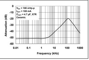
**FIGURE 2-12:** Power Supply Ripple Rejection (PSRR).
