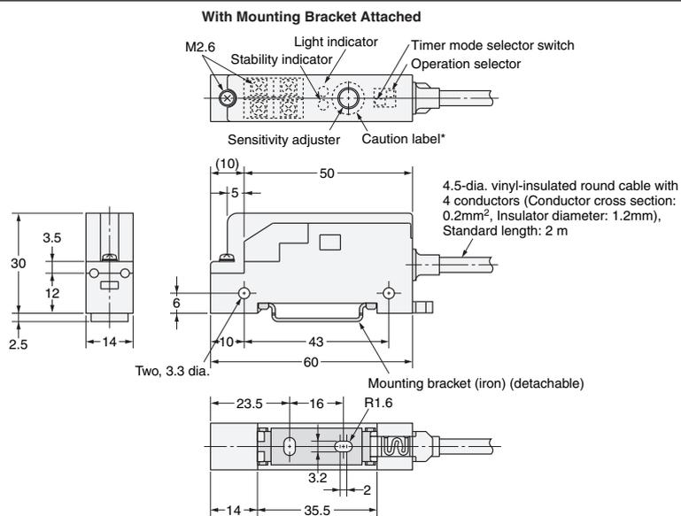
\*After adjusting the sensitivity, attach the caution label at the location indicated by
