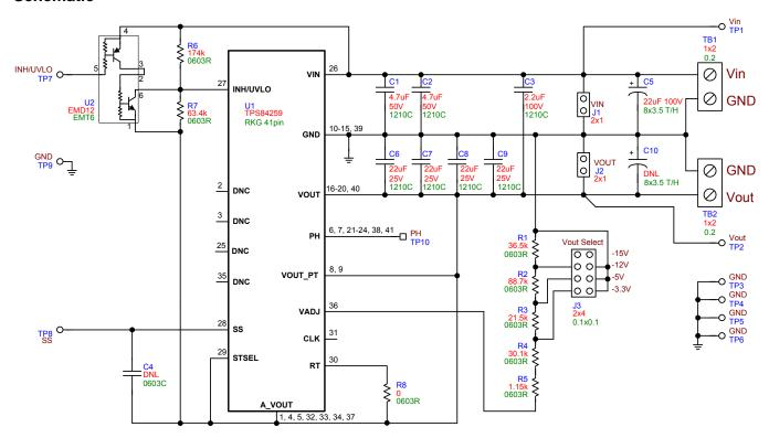
Figure 2. Schematic, TPS84259 EVM
