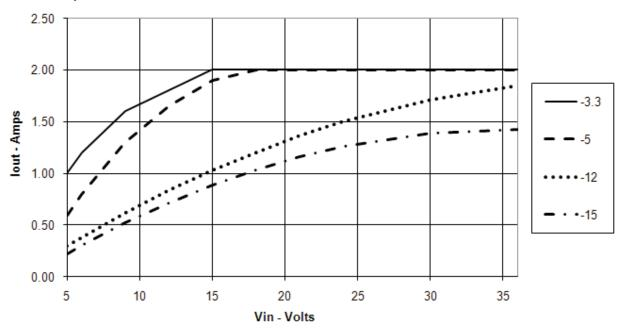
Figure 1. TPS84259 Safe Output Current
