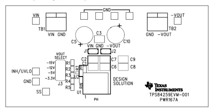
Figure 3. Top Side Components
