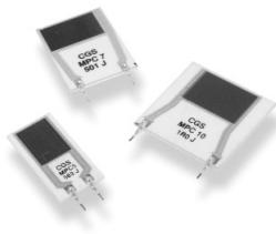
A range of non inductive thick film power resistors complementing the T0220 packaged MPR series (20 Watt heat sink styles), being vertically mounted and suitable to dissipate power from 3 Watts up to 10 Watts. Available in values from 1R0 to 200K ohms they are the ideal solution for small snubber circuits, the output side of high speed pulse generators and low inductive resistor requirements in switch mode power supplies.
