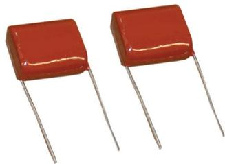
**Type DPP** radial leaded polypropylene film/foil capacitors are non-inductively wound. Very low dissipation factor and high insulation resistance contribute to excellent performance and long-term stability characteristics. Low ESR, DF and its inherent stability make **Type DPP** an ideal choice for tight tolerance, pulse and high-frequency applications.
