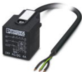
Sensor/actuator cable, 3-position, PVC, black RAL 9005, free cable end, on Valve connector A, with 1 LED, connected with Z diode, cable length: 10 m
