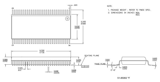
Figure 12. 56-pin SSOP (300 Mils) Package Outline, 51-85062
