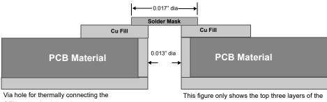
QFN to the circuit board ground plane.
