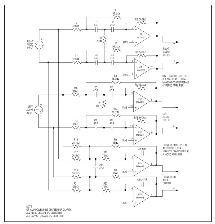
Figure 6. Fully Differential Crossover Filters
