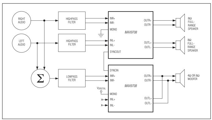
Figure 5. Multiple Amplifiers Implement a 2.1 Audio System
