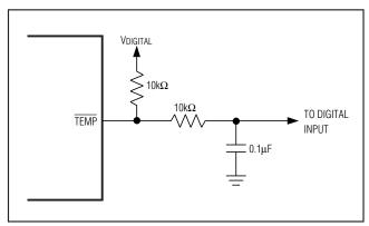
Figure 3. An RC Filter Eliminates Transient During Switching
