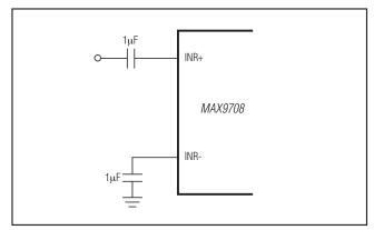
Figure 4. Single-Ended Input Connections
