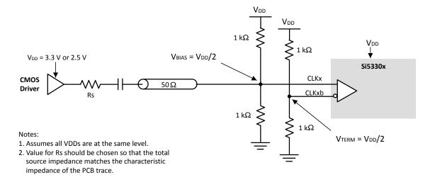
Figure 2.3. AC-Coupled, Single-Ended (LVCMOS) Input Termination
