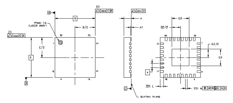
Figure 6.2. 5x5 mm 32-QFN Package Diagram Dimensions
