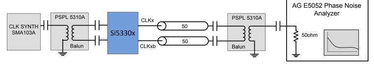
Figure 2.13. Differential Measurement Method Using a Balun
