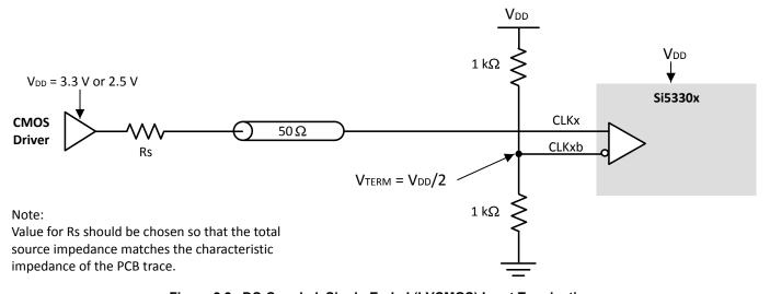
Figure 2.2. DC-Coupled, Single-Ended (LVCMOS) Input Termination
