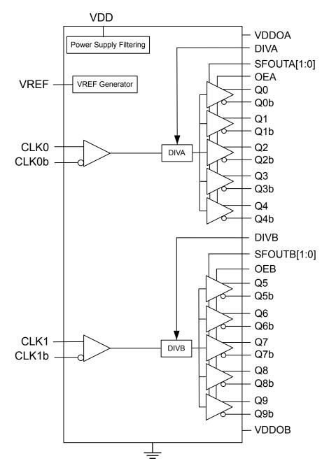
Figure 4.3. Si53303 Block Diagram
