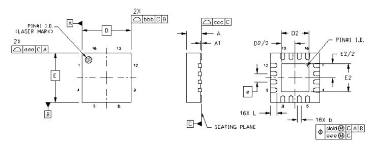
Figure 6.1. 3x3 mm 16-QFN Package Diagram Dimensions
