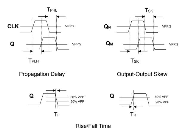
Figure 2.12. AC-Coupled Timing Waveforms
