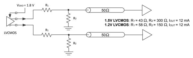
Figure 2.11. 1.5 V and 1.2 V LVCMOS Low-Voltage Output Termination
