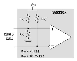
Figure 2.5. Internal Input Bias Resistors
