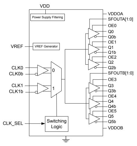
Figure 4.4. Si53304 Block Diagram
