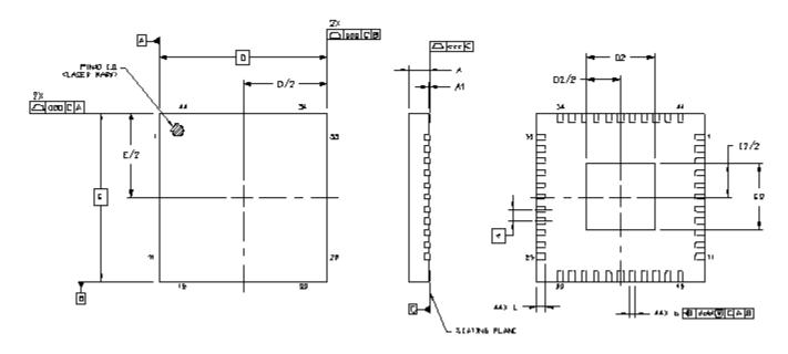
Figure 6.3. 7x7 mm 44-QFN Package Diagram Dimensions
