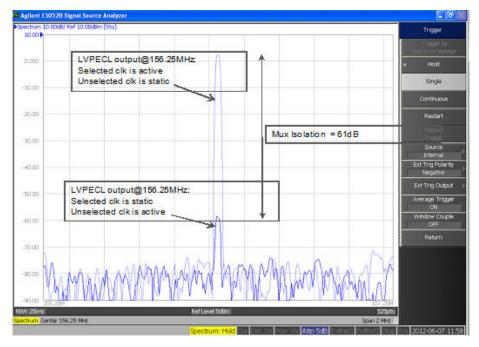
Figure 2.18. Input Mux Noise Isolation (Differential Input Clock, 44-QFN Package)
