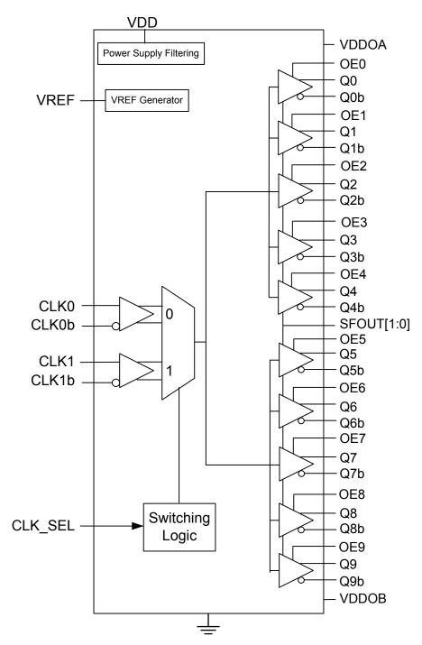
Figure 4.5. Si53305 Block Diagram
