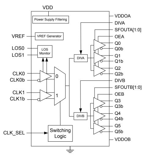
Figure 4.1. Si53301 Block Diagram
