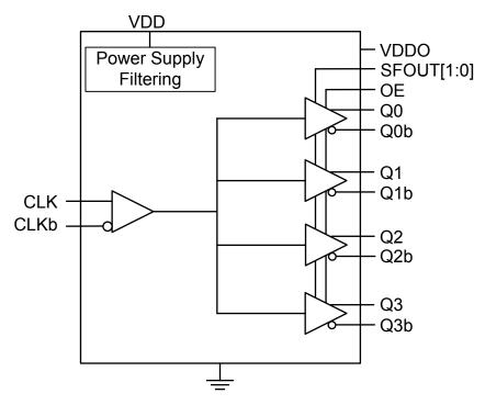
Figure 4.6. Si53306 Block Diagram
