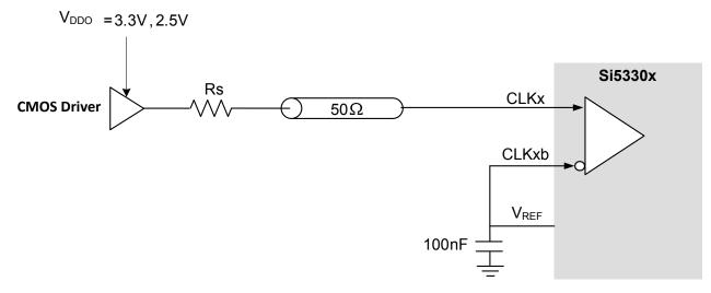
Figure 2.6. Using Voltage Reference with Single-Ended Input Clock
