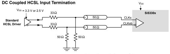
Note: 33 Ohm series termination is optional depending on the location of the receiver.
