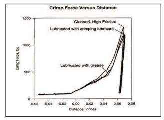
Typical Effect of Friction on Crimp Force
