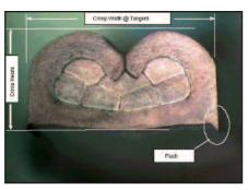
Cross Section Defining Crimp Width, Crimp Height, and Flash
