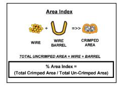
A typical design point for AI is 80%. In order to maintain the same AI, the crimp height, CH, needs to change inversely to the change of crimp width, CW, in approximately the same proportion. Thus, if the CW increases +2%, the CH needs to change approximately -2% in order to achieve the same AI design point. At first glance that may not seem significant, but in reality it can be very significant. Using another general industry design rule of the ratio of CH to CW of approximately 65%, a typical
