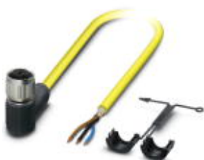
Sensor/actuator cable, 3-position, PVC, shielded, free cable end, on Socket angled M12 SPEEDCON, A-coded, cable length: 2 m
