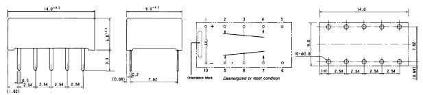
AL-D type (Double winding latching type)
