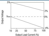
The voltage tolerance envelope shows typical load regulation characteristics for this product series. The tolerance envelope is the maximum output voltage variation due to changes in output loading.
