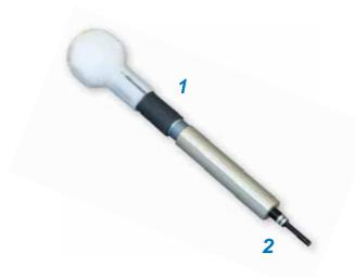
Check for properly seated contacts with this springloaded tester. Apply the tool tip to the mating end of a contact. Push on the handle until the spring compresses to the recommended force. A visual indicator shows full compression. The contact is properly retained if it is not displaced. The adjustable handle should be set to 3.2 pounds (14.2 N). The pin tip is used with #23 pin contacts. The socket tip is used with #23 socket contacts.
