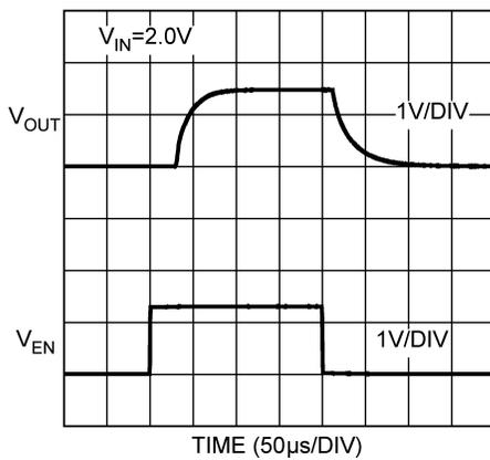
**Figure 7. Enable Characteristics**
