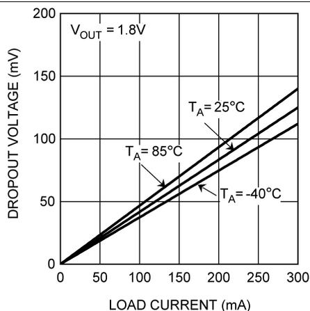
Figure 5. Dropout Voltage
