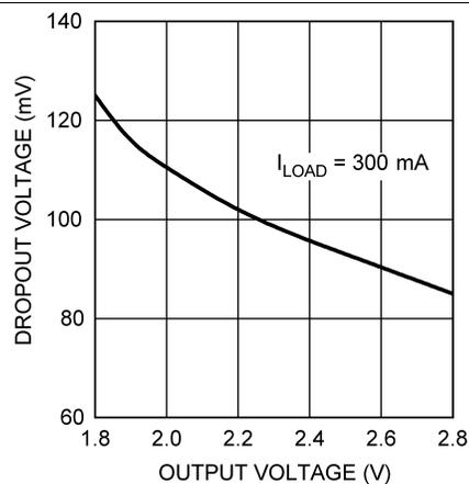
Figure 6. Dropout Voltage vs Output Voltage
