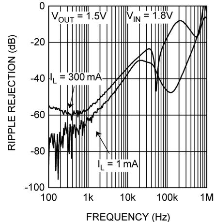
**Figure 10. Power Supply Rejection Ratio**
