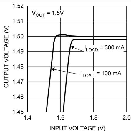
Figure 2. Output Voltage vs Minimum Input Voltage
