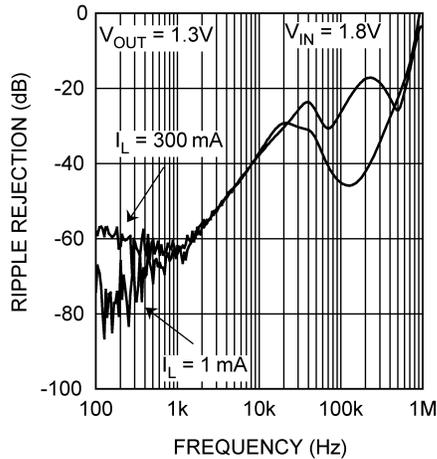
**Figure 9. Power Supply Rejection Ratio**
