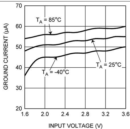
Figure 4. Ground Current vs  $V_{IN}$ ,  $I_{LOAD} = 1 \text{ mA}$
