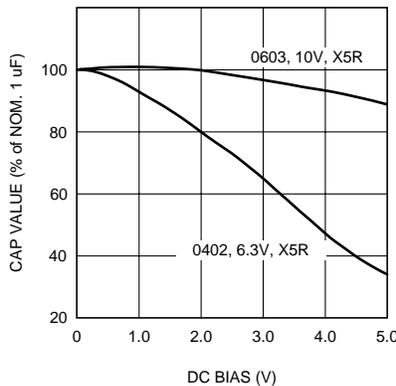
Figure 13. Effect of DC Bias on Capacitance Value
