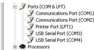
Figure 2.9 - COM Port Assignment
