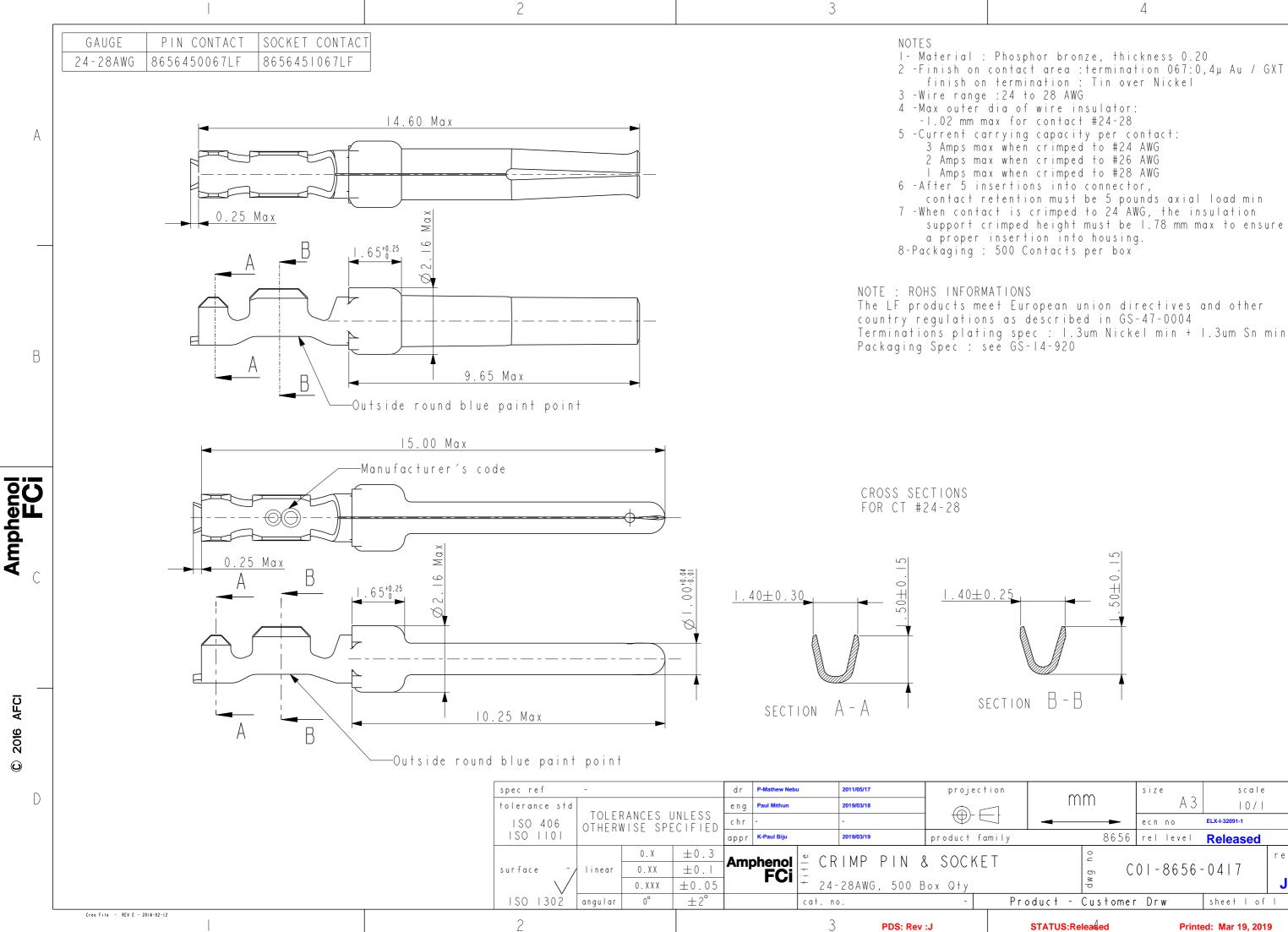
contact retention must be 5 pounds axial load min 7 -When contact is crimped to 24 AWG, the insulation support crimped height must be 1.78 mm max to ensure
