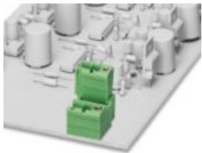
Header, Nominal current: 10 A, Rated voltage (III/2): 320 V, Number of positions: 2, Pitch: 5 mm, Color: green, Contact surface: Tin, Mounting: Wave soldering, The article can be aligned to create different nos. of positions! In combination with MVSTB or FKCV plug components, both an MVSTBW (or FKCVW) and an MVSTBR plug (or FKCVR) must be used. Combination with TMSTBP plug components is not possible!
