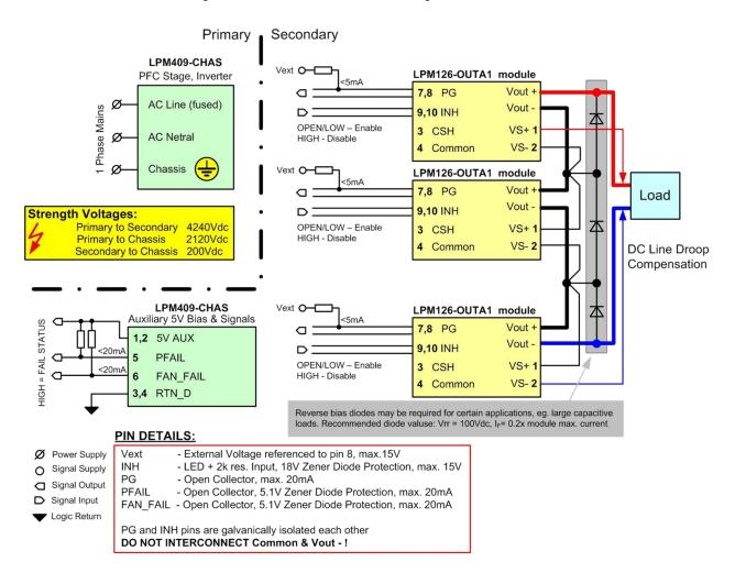
Figure 17 – LPM409 – Serial Connection Diagram for LPM126 Modules
