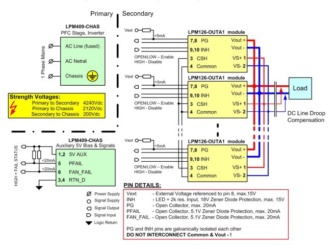
Figure 15 – LPM409 - Paralleling Connection Diagram for LPM126 Modules
