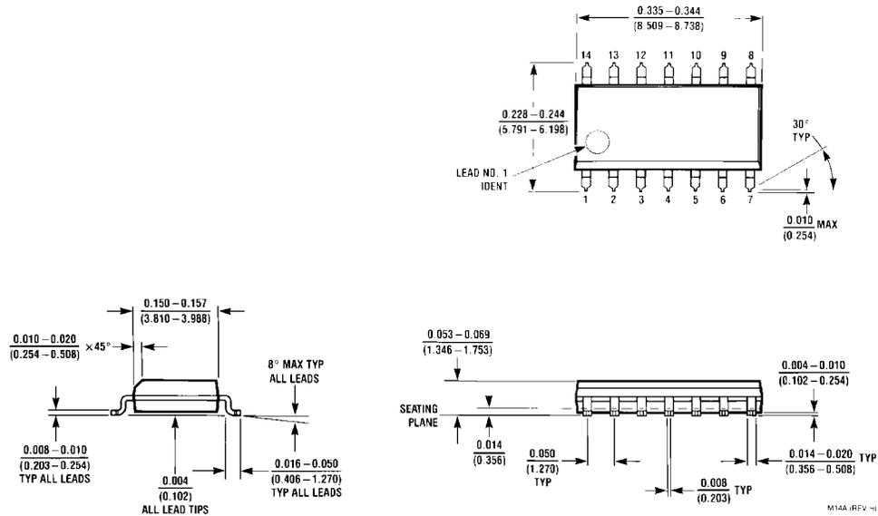
**14-Lead Small Outline Integrated Circuit (SOIC), JEDEC MS-120, 0.150" Narrow Body
